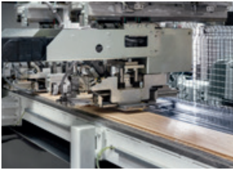
Filling knots and cracks (especially for rustic grades).
