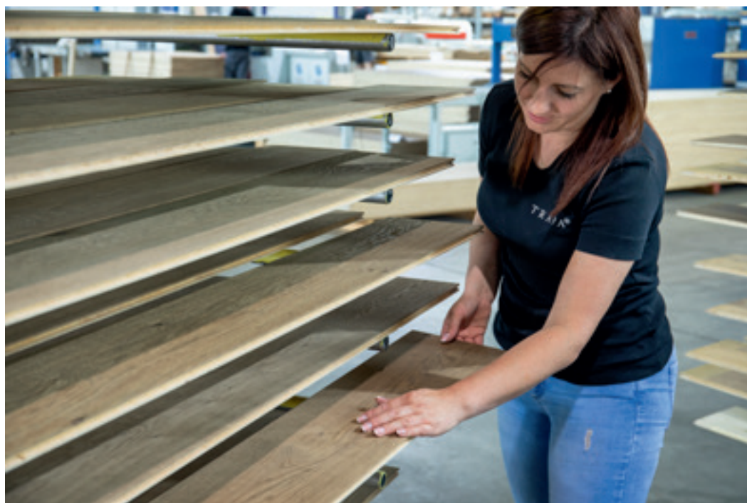
After lye-treatment each plank is air-dried on racking trolleys
