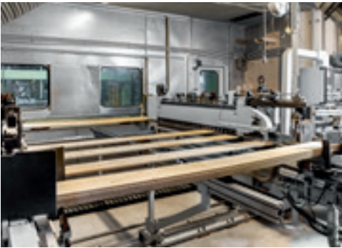
Milling of tongue and groove for tension-free connections between the floor elements.
