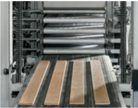
Pressing together the three tension-free solid wood layers.
