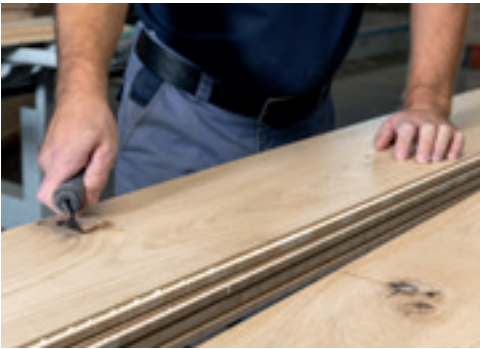
Scraping off loose branches and fibers before filling.
