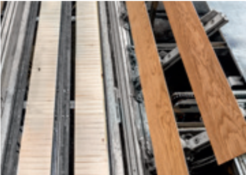
Assembling the top, core, and bottom layers of natural wood floors.
