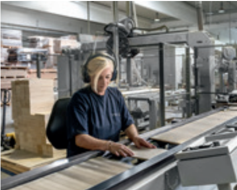
Core layer production from mountain spruce with upright annual rings.
