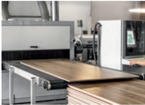
Refinement of natural wood floors with natural oil.
